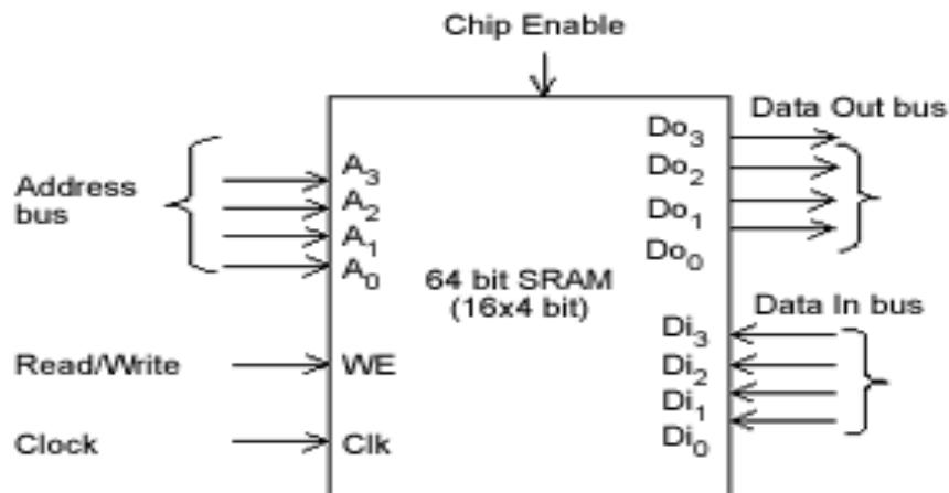
The memory block diagram is shown in above figure. It takes a few assumptions into consideration for easing the operations of the circuit. While data input pin and address pin may have any value depending on the specifications of memory used and your need, clock used in the circuit is active high.
